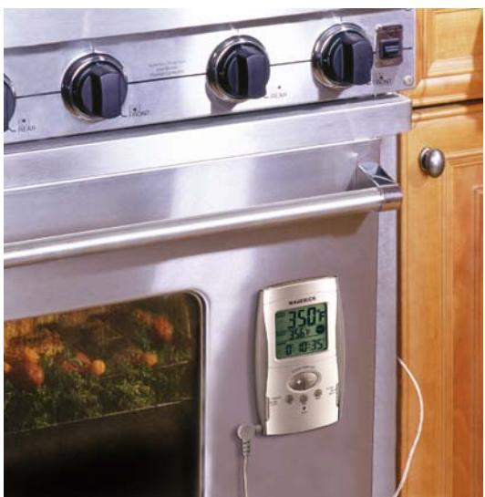
The BAKER'S OVEN THERMOMETER measures the temperature by using a probe sensor with oven rack clip, and an insulated metal wire that passes between the oven door seal back to the unit. Ovens can vary up to 50 F from the temperature you set on the dial, and every oven is different. If you don't know your oven temperature, your baking results can be poor.
